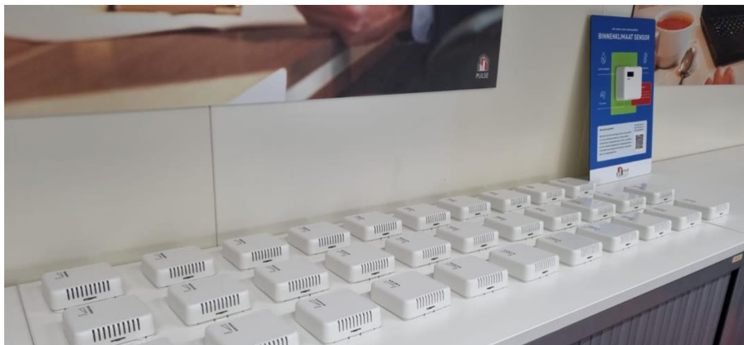
Figure 7: Indoor climate sensors placed next to each other for calibration.
